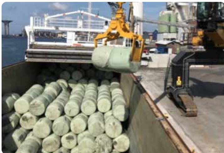
Figure 12. Baling and loading RDF in Ireland bound for Landskrona Energi Swedish Incinerator. Source: Geminor
